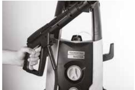
**NOTE:** never run the pressure washer with air in the hoses, which can damage the motor.
