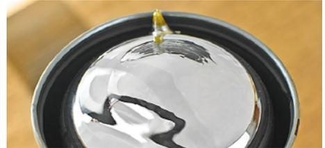
**Note:** please take care when handling the insulated support. If it is damaged, the flask loses its thermal efficiency. Do not remove the sticker that is located near the capillary, it serves for product traceability.
