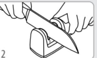
In both cases, move the knife blade from its end to near the handle, employing light pressure on the blade between the sharpener's rollers. Repeat the movement as many times as necessary. Edge maintenance sharpening, position 2 only, can be carried out before each use of the knife.
